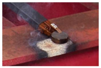
Heating is an important part of frame straightening
