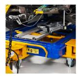
The measuring slide mounts and moves on the Measuring Bridge, which has microscopic markings in its rails to enable the measuring head beneath the slide to determine its horizontal position. Available in 4, 5 & 6 meter lengths.
