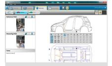
In Absolute and Comparative measuring modes it is possible to describe, with photos and in text, how the different points have been measured.
