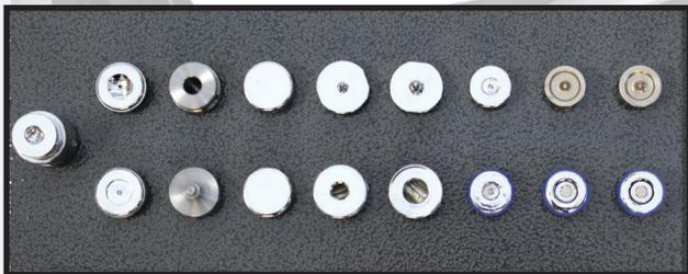
The PR-5 self-piercing rivets join two or more pieces of material with the use of extreme pressure and precision machined punch and die sets. The punches are magnetic to hold the rivets in place, making operation quick and easy. The dies complete the process and prevent the rivet from punching through the last layer of material. This allows you to join different materials such as: aluminum, steel, plastic and more.
