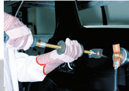
Spot hammer welding
