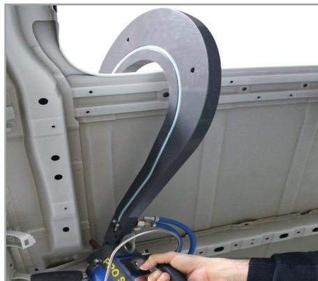
For deeper needs use the Pro Spot extension U-Arms (508mm - 600mm). They are self aligning and quick to install.
