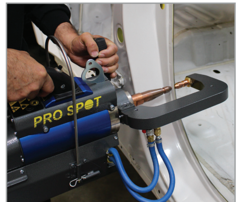
Spot welding of quarter panel using C-Arm.
