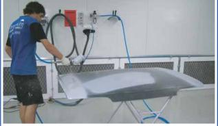
The Lowbake Extraction Wall Prep Area is a simple low cost extraction unit for sanding as well as a preparation area. The unit is fitted with paint pocket polyester exhaust filters to stop dust emissions. The large span filters allow for work to be carried out on varying sizes of parts.
