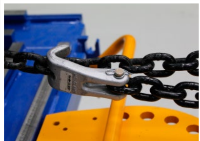
Strong pulling capability with the 10-ton chain kit
