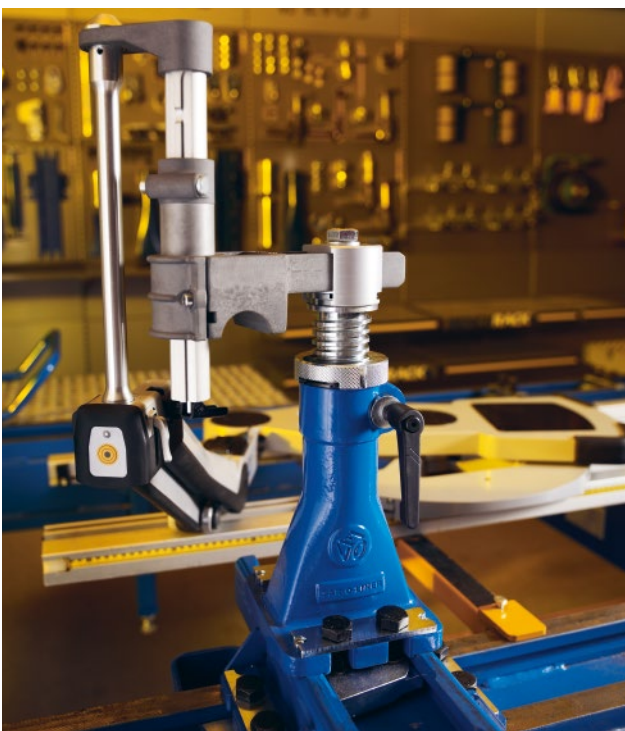
EVO universal fixturing system with Car-O-Tronic electronic measuring system
