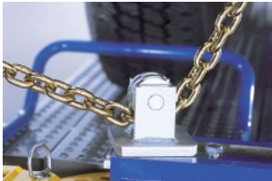
Down pulls may be quickly executed with the D91 support system
