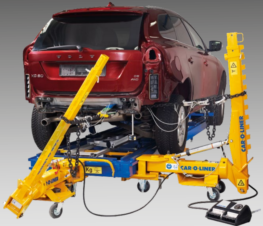
Simultaneous multiple pulling capabilities with our powerful 10-ton draw aligners that can pull from almost any angle, 360° around the vehicle
