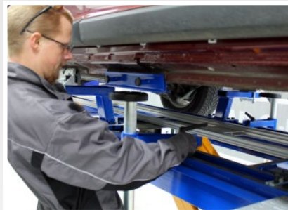
Exclusive pillar jacks and threshold (rocker) supports make mounting of vehicles fast, safe and easy
