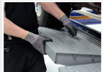
Removable ramp sections lift out easily to allow better access to the vehicle
